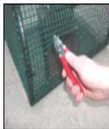
Hog ring tools for rigging, single ring or magazine fed.
