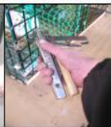
Hog ring tools for rigging, single ring or magazine fed.
